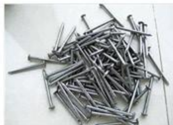
普通圆钉 COMMON NAILS SIZE: DIA: BWG5-BWG20 LENGTH: 1/2", 1", 1.5", 2", 2.5", 3", 3.5", 4", 5", 6", 7", 8"
